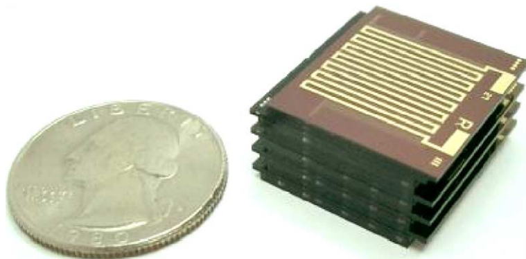
Fig. 2. Photograph of the multi-layered microreactor.
